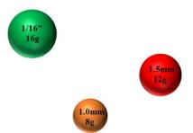
50% a reduction in ring mass equals a 50% reduction in the inertia force on that ring. In addition to the reduced reciprocating mass, the inertia reduction from lighter rings allows for operation at higher RPMs with less ring flutter, further increasing the ring to piston groove seal.
