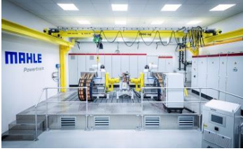
Electric drives are tested under real conditions on the electric motor test bench in Fellbach/Germany.
