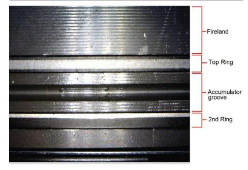
Engine assembly mistakes. This is a close-up look at the top two rings on a piston from an engine that was smoking, indicating excessive oil consumption.
