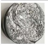
Over-revved/dropped valve. When a valve has dropped there's no question about the cause of the carnage.
