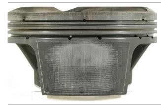
Excess engine temperature. In this situation the engine cooling system is the culprit, though the piston initially appears to be to blame.
