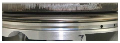
Ring Land Erosion. Vertical scoring/ erosion above a piston's top ring groove is another symptom of faulty combustion, specifically detonation.
