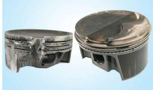
pitting and erosion evident just to the right of the valve pockets.
