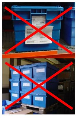
• To prevent parts from getting mixed up in the production process, only the currently valid shipping/parts identification label must be used on the container.
