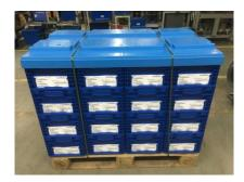
• For MULTIPACK, the plastic strap must be routed through the grooves in the lid (not the hinge).
