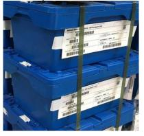
Basically, size of labels (VDA 4902, VDA4994) should be aligned to size of KLT
